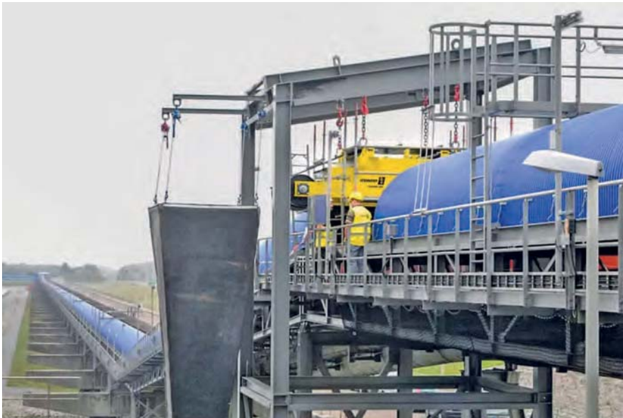
Air-cooled magnet options include the STEINERT UME with an extremely strong and far-reaching magnetic field designed for high bed depths and small tramp metal
